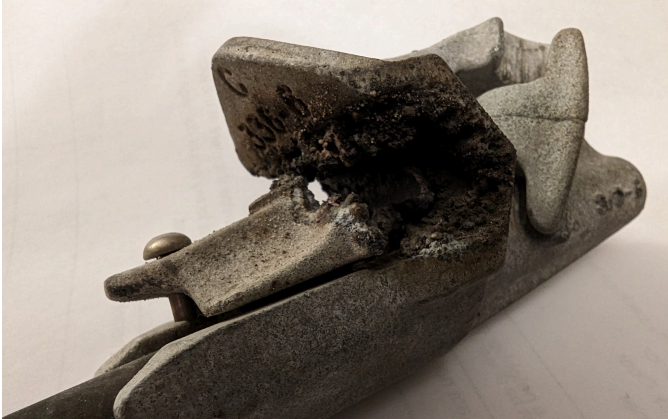
Fig. 3: Arcing clamp detected and repaired before catastrophic failure
