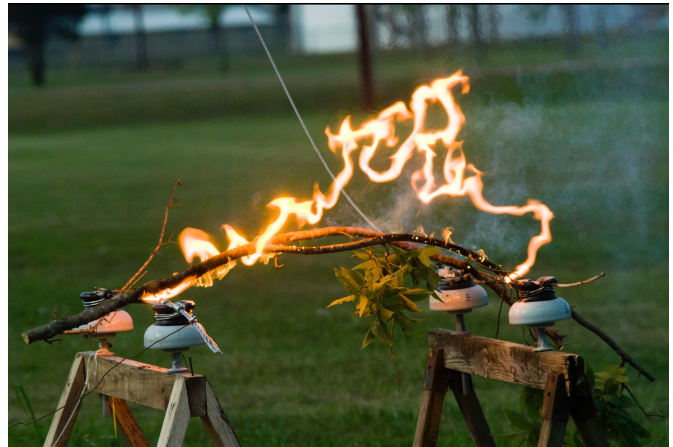
Fig. 2: Flashover produced by vegetation contact.
